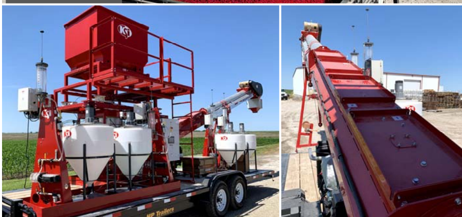
Gentle Seed Handling/Mixing — Static Mixing Belt Conveyor
